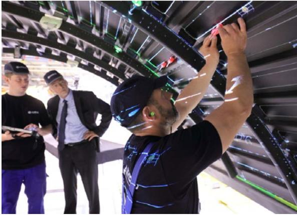
SINCE 2011, AIRBUS CORPORATION has been introducing a Smart Augmented Reality Tool for quality control in its production. Tablets with special sensors and software impose schemes on the real objects, providing immediate access to databases that contain all the necessary information. At the moment, over 1,000 Airbus employees are using the Smart Augmented Reality Tool in their work.
